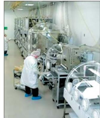
**Figure 2.** An Xcellerex FlexFactory installation for vaccine production. (Source: MediVas)
